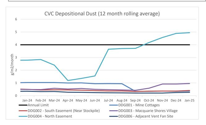
A 12-month rolling average of depositional dust concentrations has been presented above. Dust Gauges DDG001, DDG002, DDG003 and DDG004 are located within a closer proximity to Chain Valley Colliery and DDG006 is positioned in a location representative of the Chain Valley Colliery ventilation fan site at Summerland Point.
